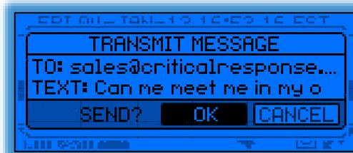
Once you select OK, the message is placed into the M1503 transmit queue, where it will wait for a few seconds until transmitted to the network. While messages are in queue, the number of pending transmissions will appear next to the **Sent Messages** menu item on the **Main Menu** page. Once all pending messages are successfully transmitted, this count will vanish.
