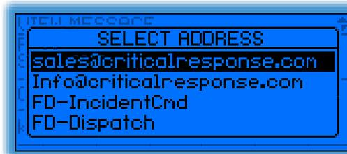
Selecting the **Forward** action from the message options pop-up menu brings up a second pop-up window displaying your list of canned addresses. You may navigate through the list using the **Up** and **Down** buttons, and select an address by pressing the **Select** button. This will forward the message to the selected address. You may also return to the **View Message** page at any point, without forwarding the message, by pressing **Escape** button.
