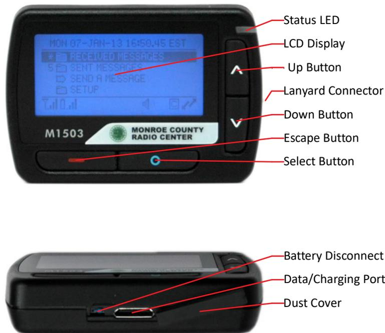
Your M1503 consists of a digital radio, CPU, LCD display, four buttons, a speaker, a status LED, and a data/charging port, enclosed together in a durable polycarbonate housing. It also comes with a belt holster, bungee, and charging cable, along with an optional charging/programming dock and wall adapter.
