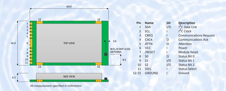
The **M1402** Endpoint Transceiver enables OEM objects to connect to an IOCAST cloud and communicate with backend applications.
