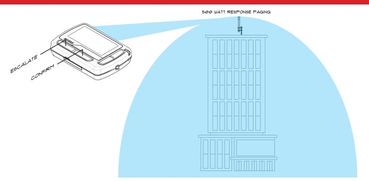
Response paging uses one high power antenna for reliable, uniform coverage. Users receive notifications anywhere within the hospital, and simple user equipment displays messages without disrupting workflow or distracting the recipient.
