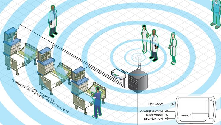
Response paging systems use two synchronized radio channels: a high-power channel to send messages, and a medium-power channel to receive confirmation and responses. One antenna provides reliable coverage to an entire hospital complex.
